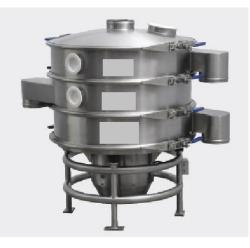
Rubber mounted suspension without spring – Acceptable. Open frame design with no sheet metal enclose – Acceptable. <u>Non acceptable item:</u>
